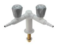
TECHNICAL FEATURES Media: Vacuum Minimum pressure: down to 1 mbar Fluid identification: EN 13792 Design: DIN 12918-3 Nozzle: DIN 12898 Inlet: Male thread ISO 228 G3/8" x 60 mm
