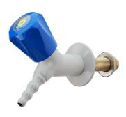
TECHNICAL FEATURES Media: Compressed Air Maximum pressure: 10 bar Fluid identification: EN 13792 Design: DIN 12918-3 Nozzle: DIN 12898 Inlet: Male thread ISO 228 G3/8" x 60 mm
