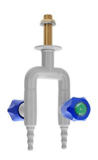
TECHNICAL FEATURES Media: Dry Services Maximum pressure: 10 bar, according to fluid Fluid identification: EN 13792 Design: DIN 12918-3 Nozzle: DIN 12898 Inlet: Male thread ISO 228 G3/8" x 60 mm
