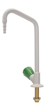
TECHNICAL FEATURES Media: Water Maximum pressure: 10 bar Maximum temperature: 65° C Fluid identification: EN 13792 Design: DIN 12918-1 Nozzle: DIN 12898 Inlet: Male thread ISO 228 G3/8" x 60 mm
