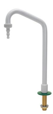
TECHNICAL FEATURES Media: Water Maximum pressure: 10 bar Design: DIN 12918-1 Nozzle: DIN 12898 Inlet: Male thread ISO 228 G3/8" x 60 mm
