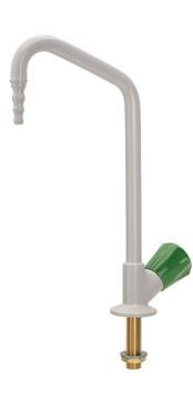
TECHNICAL FEATURES Media: Water Maximum pressure: 10 bar Maximum temperature: 65° C Fluid identification: EN 13792 Design: DIN 12918-1 Nozzle: DIN 12898 Inlet: Male thread ISO 228 G3/8" x 60 mm
