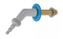
TECHNICAL FEATURES Media: Water, Burning Gas, Dry Services Maximum pressure: 10 bar Design: DIN 12918 Nozzle: DIN 12898 Inlet: Male thread ISO 228 G3/8" x 60 mm
