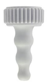
TECHNICAL FEATURES Media: All Services Nozzle: DIN 12898 Material: Polypropylene, light grey colour RAL 7035 Includes O'Ring Connection: Female thread ISO 228 G1/2"
