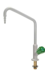
TECHNICAL FEATURES Media: Water Maximum pressure: 10 bar Maximum temperature: 65° C Fluid identification: EN 13792 Design: DIN 12918-1 Nozzle: DIN 12898 Inlet: Male thread ISO 228 G1/2" x 60 mm
