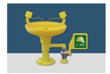
GENERAL FEATURES MATERIALS: Galvanized steel piping. Brass fittings. ANTICORROSIVE PLASTIC COATING: Polyamide with a thickness of 250-300 microns, in high-visibility yellow color. WATER INLET: Male thread ISO 228 G1/2" WATER INLET PRESSURE: Recommended 2 bar / Min. 1.5 bar / Max. 8 bar
