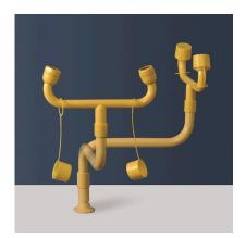
GENERAL FEATURES MATERIALS: Brass fittings. ANTICORROSIVE PLASTIC COATING: Polyamide with a thickness of 250-300 microns, in high-visibility yellow color. WATER INLET: Male thread ISO 228 G1/2" WATER INLET PRESSURE: Recommended 3 bar
