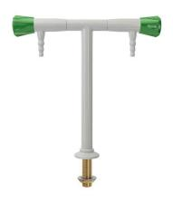
TECHNICAL FEATURES Media: Water Maximum pressure: 10 bar Maximum temperature: 65° C Fluid identification: EN 13792 Design: DIN 12918-1 Nozzle: DIN 12898 Inlet: Male thread ISO 228 G1/2" x 60 mm
