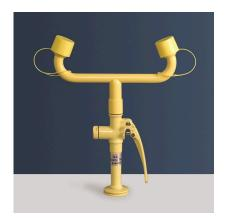
GENERAL FEATURES MATERIALS: Flexible hose in stainless steel. Brass fittings. ANTICORROSIVE PLASTIC COATING: Polyamide with a thickness of 250-300 microns, in high-visibility yellow color. WATER INLET: Female thread ISO 228 G1/2" WATER INLET PRESSURE: Recommended 2 bar / Min. 1.5 bar / Max. 8 bar
