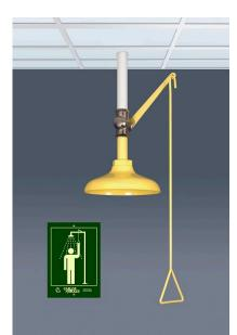
GENERAL FEATURES MATERIALS: Galvanized steel piping. Brass fittings. ANTICORROSIVE PLASTIC COATING: Polyamide with a thickness of 250-300 microns, in high-visibility yellow color. WATER INLET: Male thread ISO 228 G1" WATER INLET PRESSURE: Recommended 2 bar / Min. 1.5 bar / Max. 8 bar
