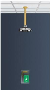
GENERAL FEATURES MATERIALS: Galvanized steel piping. Brass fittings. ANTICORROSIVE PLASTIC COATING: Polyamide with a thickness of 250-300 microns, in high-visibility yellow color. WATER INLET: Male thread ISO 228 G1" WATER INLET PRESSURE: Recommended 2 bar / Min. 1.5 bar / Max. 8 bar
