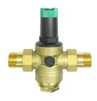
The valve reduces a high water supply pressure to a constant lower pressure. The variations in the inlet pressure do not influence the outlet pressure, it is balanced.
