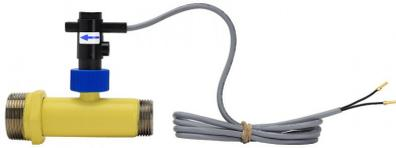
*Installed in the water inlet, when the Shower / Eyewash is activated the flowswitch sends an electrical signal to another device, allowing to alert first aid team.*
