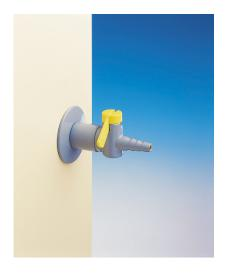
TECHNICAL FEATURES Media: Burning Gas Maximum pressure: 0.2 bar Design: DIN 12918-2 Inlet: Male thread ISO 228 G3/8" x 60 mm
