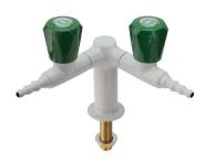
TECHNICAL FEATURES Media: Water Maximum pressure: 10 bar Maximum temperature: 65° C Fluid identification: EN 13792 Design: DIN 12918-1 Nozzle: DIN 12898 Inlet: Male thread ISO 228 G3/8" x 60 mm
