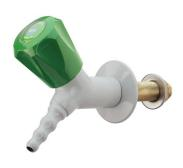
TECHNICAL FEATURES Media: Water Maximum pressure: 10 bar Maximum temperature: 65° C Fluid identification: EN 13792 Design: DIN 12918-1 Nozzle: DIN 12898 Inlet: Male thread ISO 228 G3/8" x 60 mm
