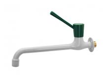
TECHNICAL FEATURES Media: Water Maximum pressure: 10 bar Maximum temperature: 65° C Fluid identification: EN 13792 Design: DIN 12918-1 Aerator: UNE-EN 246 Inlet: Male thread ISO 228 G1/2" x 12 mm
