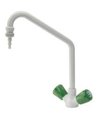
TECHNICAL FEATURES Media: Water Maximum pressure: 10 bar Maximum temperature: 65° C Fluid identification: EN 13792 Design: DIN 12918-1 Nozzle: DIN 12898 Inlet: Two AISI 304 braided flexible hoses with female thread ISO 228 G3/8"
