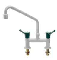
TECHNICAL FEATURES Media: Water Maximum pressure: 10 bar Maximum temperature: 65° C Fluid identification: EN 13792 Design: DIN 12918-1 Aerator: UNE-EN 246 Inlet: Two male threads ISO 228 G1/2" x 60 mm
