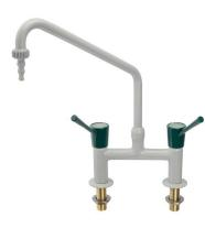
TECHNICAL FEATURES Media: Water Maximum pressure: 10 bar Maximum temperature: 65° C Fluid identification: EN 13792 Design: DIN 12918-1 Nozzle: DIN 12898 Inlet: Two male threads ISO 228 G1/2" x 60 mm
