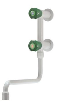
TECHNICAL FEATURES Media: Water Maximum pressure: 10 bar Maximum temperature: 65° C Fluid identification: EN 13792 Design: DIN 12918-1 Aerator: UNE-EN 246 Inlet: Two male threads ISO 228 G3/8" x 60 mm
