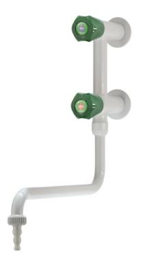
TECHNICAL FEATURES Media: Water Maximum pressure: 10 bar Maximum temperature: 65° C Fluid identification: EN 13792 Design: DIN 12918-1 Nozzle: DIN 12898 Inlet: Two male threads ISO 228 G3/8" x 60 mm
