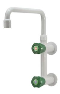
TECHNICAL FEATURES Media: Water Maximum pressure: 10 bar Maximum temperature: 65° C Fluid identification: EN 13792 Design: DIN 12918-1 Aerator: UNE-EN 246 Inlet: Two male threads ISO 228 G3/8" x 60 mm
