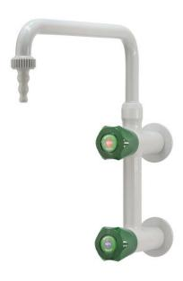
TECHNICAL FEATURES Media: Water Maximum pressure: 10 bar Maximum temperature: 65° C Fluid identification: EN 13792 Design: DIN 12918-1 Nozzle: DIN 12898 Inlet: Two male threads ISO 228 G3/8" x 60 mm
