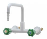
TECHNICAL FEATURES Media: Water Maximum pressure: 10 bar Maximum temperature: 65° C Fluid identification: EN 13792 Design: DIN 12918-1 Nozzle: DIN 12898 Inlet: Two male threads ISO 228 G1/2" x 60 mm
