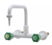
TECHNICAL FEATURES Media: Water Maximum pressure: 10 bar Maximum temperature: 65° C Fluid identification: EN 13792 Design: DIN 12918-1 Nozzle: DIN 12898 Inlet: Two male threads ISO 228 G1/2" x 60 mm
