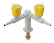
TECHNICAL FEATURES Media: Burning Gas Maximum pressure: 0.2 bar Fluid identification: EN 13792 Design: DIN 12918-2 Nozzle: DIN 12898 Inlet: Male thread ISO 228 G3/8" x 60 mm
