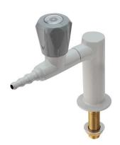
TECHNICAL FEATURES Media: Vacuum Minimum pressure: down to 1 mbar Fluid identification: EN 13792 Design: DIN 12918-3 Nozzle: DIN 12898 Inlet: Male thread ISO 228 G3/8" x 60 mm
