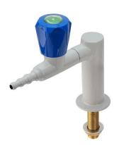
TECHNICAL FEATURES Media: Dry Services Maximum pressure: 10 bar, according to fluid Fluid identification: EN 13792 Design: DIN 12918-3 Nozzle: DIN 12898 Inlet: Male thread ISO 228 G3/8" x 60 mm
