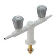
TECHNICAL FEATURES Media: Vacuum Minimum pressure: down to 1 mbar Fluid identification: EN 13792 Design: DIN 12918-3 Nozzle: DIN 12898 Inlet: Male thread ISO 228 G3/8" x 60 mm
